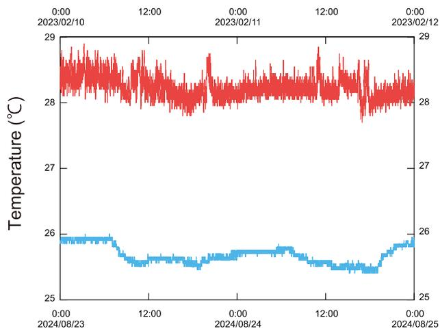
Fig. 3. Room temperature in EH2 before (red) and after (blue) removal of motor drivers.
