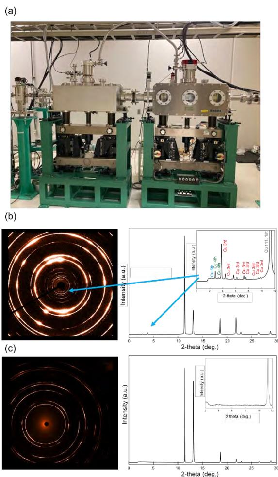
Fig. 1. (a) Mirror chamber located in the optical hutch. (b), (c) 2D and 1D XRD patterns of copper foil acquired without and with harmonic rejection mirror, respectively.
