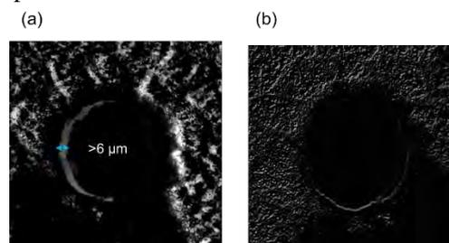
Fig. 2. Images of a  $60\text{-}\mu\text{m}$ -diameter pinhole mounted on the sample stage (a) before and (b) after the floor was repaired.
